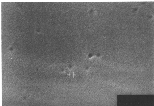
Figure 8. SEM micrograph of glow-discharge treated PC membrane with a pore size of 0.05 \mu\text{m} (Mag: X 60K).
