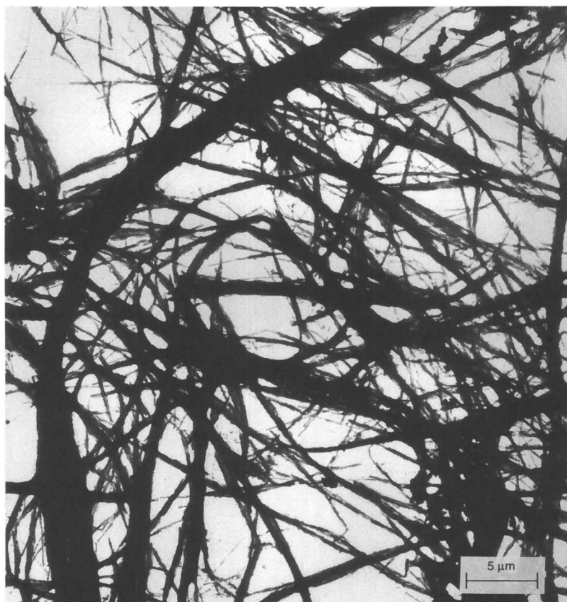
Figure 2. TEM of cylindrical microstructures formed from a 1:1 ratio of 1 and 2.
